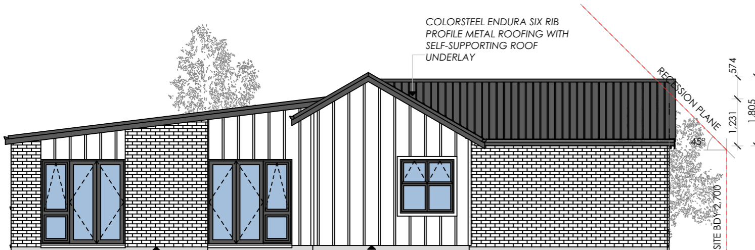
ELEVATION 1 (SOUTHERN) 70 SERIES CLAY BRICK VENEER EXTERIOR CLADDING (PAINTED) H3.1 PLY BOARD & BATTEN CLADDING ON 20mm VENTED CAVITY SYSTEM
