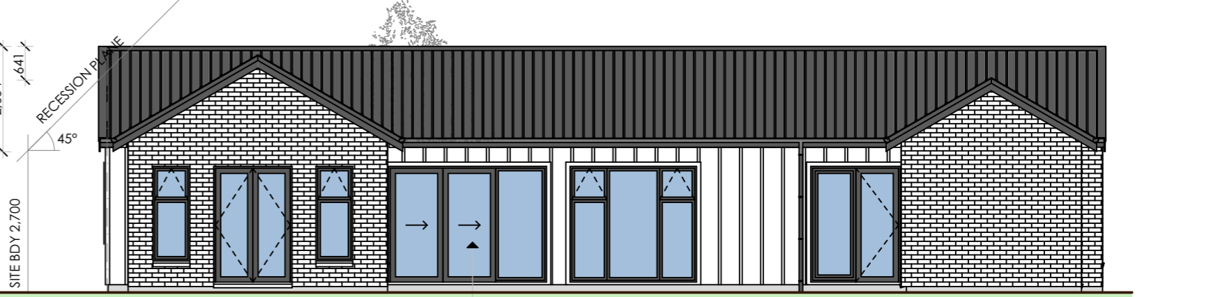
ELEVATION 4 (EASTERN) DOUBLE GLAZED P.C. ALUMINIUM JOINERY
